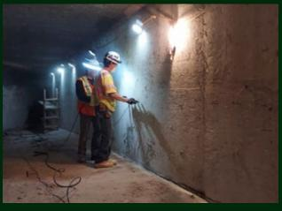
Post-tension void detection using sonic/ultrasonic testing and ground penetrating radar, Orangethorpe, CA
