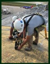
Impact echo/pulse velocity testing of a hangar at the Kansas City Airport
